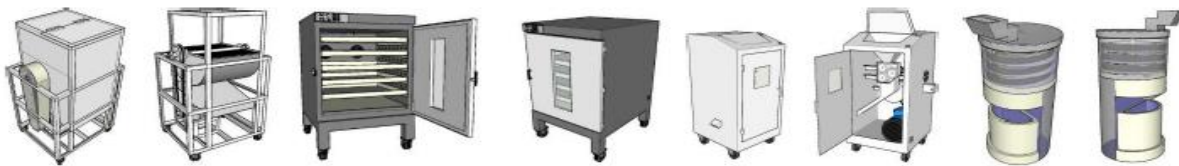
Picture Description: Isometric view of machine design of 1) coffee demucilager, 2) dryer, 3) huller, and 4) sorter
