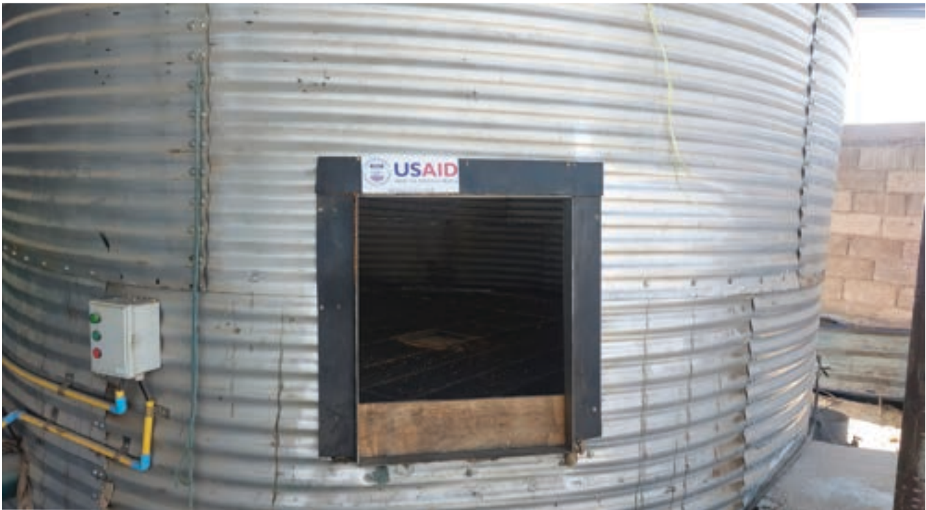
Batch dryer installed beside a trader's maize shed
