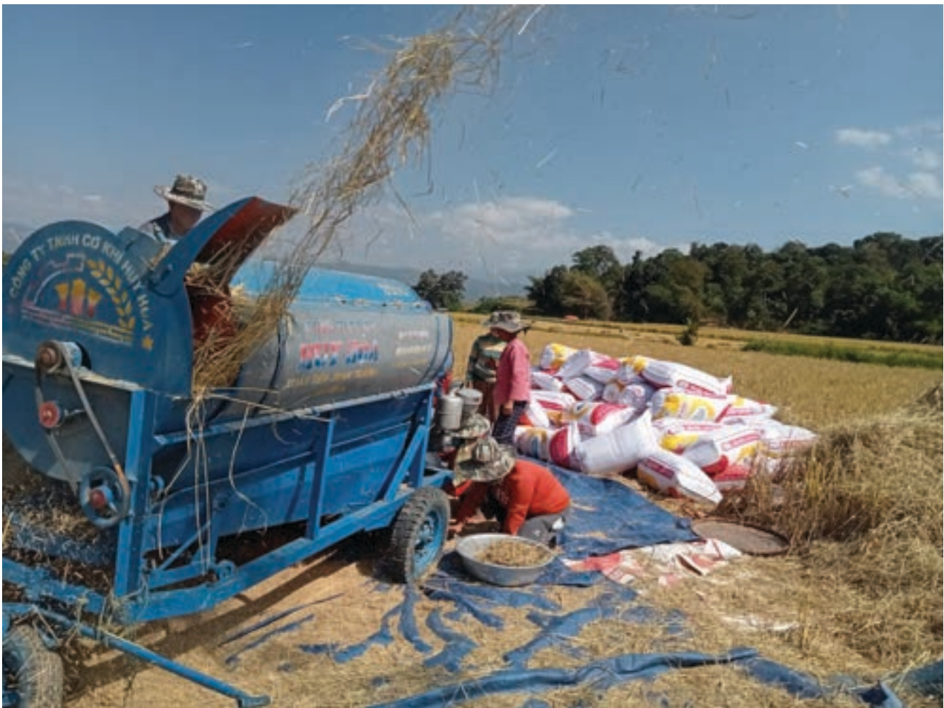
Large rice thresher separating paddy from stalks in the field
